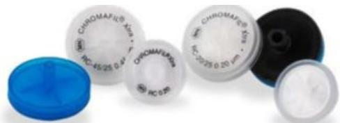
Syringe filters, CHROMAFIL Xtra RC, Inside the syringe filter a regenerated cellulose is used as membrane material. The hydrophilic RC membrane is suitable for aqueous and organic – aqueous liquids, i.e. polar and medium polar sample solutions and shows a low binding capacity for proteins. Labeled for method validation and certification. All CHROMAFIL filters are autoclavable (121 °C and 1.1 bar for 30 min)!
