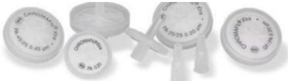
Syringe filters, labeled, CHROMAFIL Xtra PA, Inside the syringe filter polyamide is used as membrane material. The rather hydrophilic PA membrane is suitable for filtration of medium polar organic-aqueous liquids.
