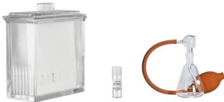
If you would like to coat TLC plates yourself, we offer suitable adsorbents for thin layer chromatography. In addition to our ready-to-use layers in TLC and HPTLC, the product range also includes accessories.
