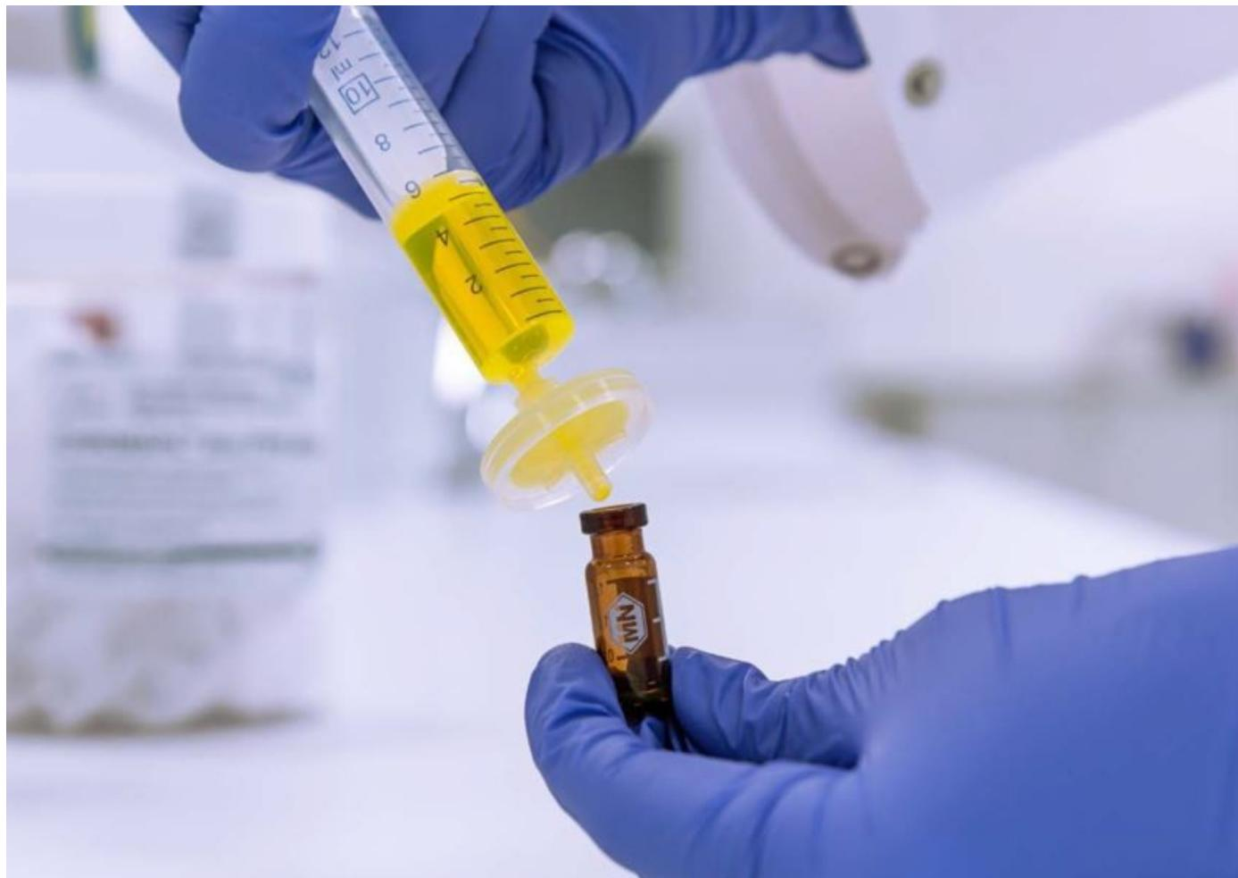
CHROMAFIL filtration products avoid contamination of sensitive instrumentation and increase the lifetime of columns and equipment. We offer different membranes (e.g., PTFE, RC, nylon) in syringe filters, filter cartridges and filter 96well plates for rapid purification and removal of particles.
