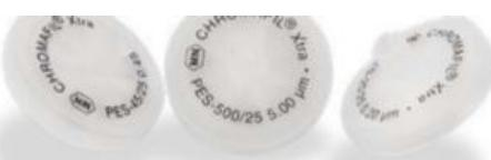
Syringe filters, CHROMAFIL Xtra PES, Inside the syringe filter polyethersulfone is used as membrane material. The hydrophilic PES membrane is suitable for aqueous and slightly organic liquids. This filter shows a good stability against acids and bases as well as a very low adsorption for pharmaceuticals and proteins. Labeled for method validation and certification. All CHROMAFIL filters are autoclavable (121 °C and 1.1 bar for 30 min)!
