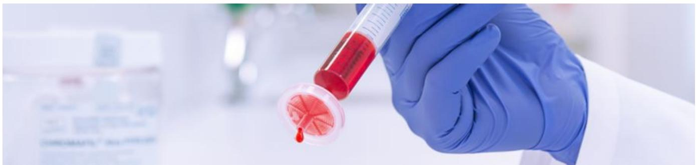
CHROMAFIL and CHROMAFIL Xtra syringe filters increase the lifetime of columns and equipment by removal of solid particles. Different membranes (e.g., PTFE, RC, nylon) and pore sizes are used for rapid purification of your samples.
