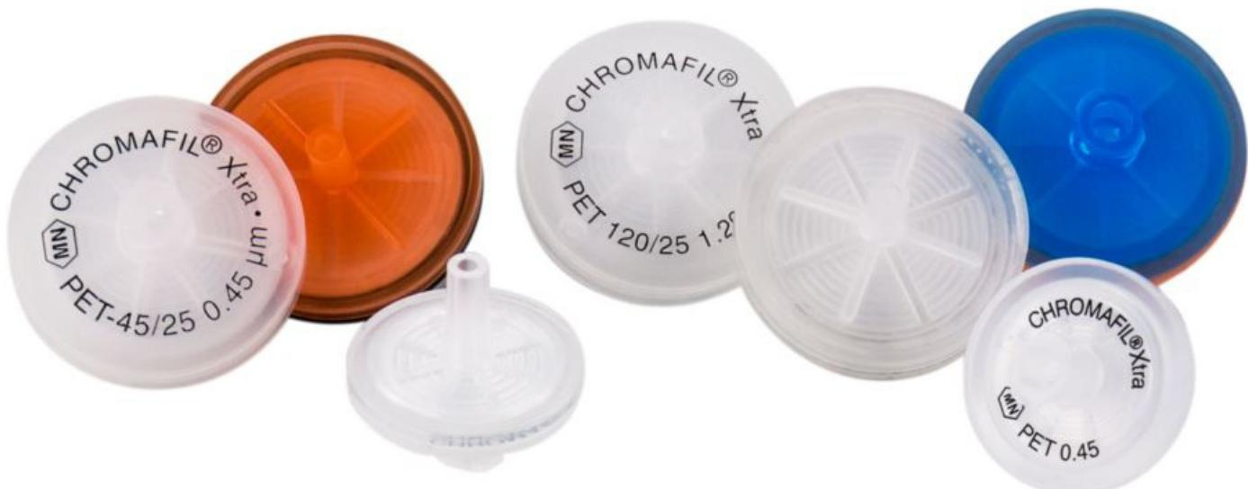
Syringe filters, color coded, CHROMAFIL PET, Inside the syringe filter polyester (polyethylene terephthalate) is used as membrane material. The hydrophilic multipurpose PET membrane is for polar as well as nonpolar solvents. It is the HPLC filter, especially suited for mixtures of water and organic solvents. It is not cytotoxic, does not inhibit the growth of microorganisms and higher cells. All CHROMAFIL filters are autoclavable (121 °C and 1.1 bar for 30 min)!
