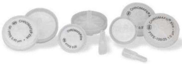
Syringe filters, labeled, CHROMAFIL Xtra PTFE, Inside the syringe filter polytetrafluoroethylene is used as membrane material. The hydrophobic PTFE membrane is very resistant towards all kinds of solvents as well as acids and bases. Flushing with alcohol, followed by water, makes the originally hydrophobic membrane more hydrophilic.
