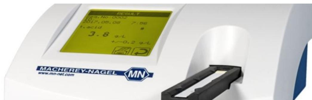
The QUANTOFIX Relax is the ideal device for the objective evaluation of our QUANTOFIX and pH-Fix test strips. It combines the simplicity of test strips with the safety of instrumental analysis and thus the best out of these two worlds. The QUANTOFIX Relax does not require any special strips, but evaluates the normal pH-Fix and QUANTOFIX test strips. Therefore entrance into instrumental analysis is very simple; the same strip can be used for visual and instrumental evaluation.
