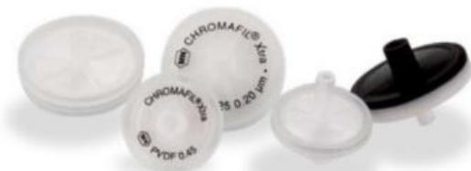
Syringe filters, CHROMAFIL Xtra PVDF, Inside the syringe filter polyvinylidene difluoride is used as membrane material. The hydrophilic PVDF membrane is suitable for filtration of 100 % aqueous samples, water-soluble oligomers and polymers like proteins. Extremely low binding capacity for proteins. Labeled for method validation and certification. All CHROMAFIL filters are autoclavable (121 °C and 1.1 bar for 30 min)!
