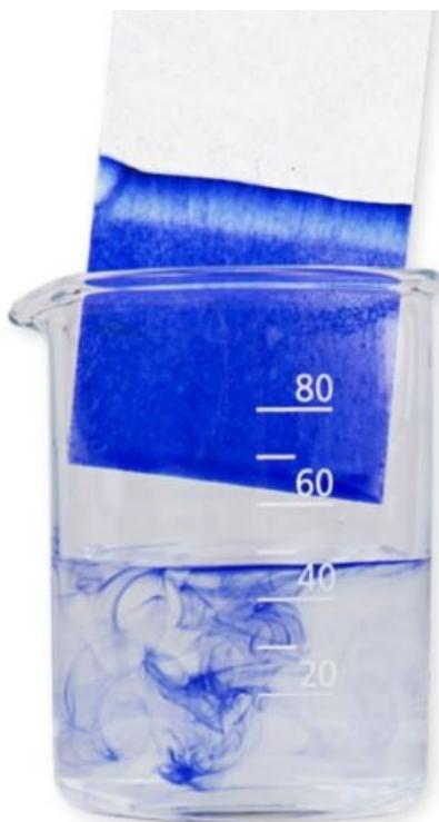
Qualitative test papers come without a color scale. With little effort, the presence of ions and other substances can be detected. The test papers change their color when the concentration is above the specified limit of detection.
