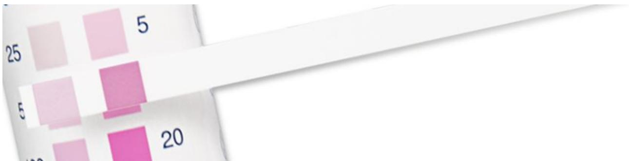
Test papers and test strips for semi quantitative analysis are extremely simple to handle. They are based on the principle of "Dip & Read". They are available for a variety of parameters and comply with all requirements of a modern rapid test. The evaluation of these tests is carried out by a comparison with a color scale.
