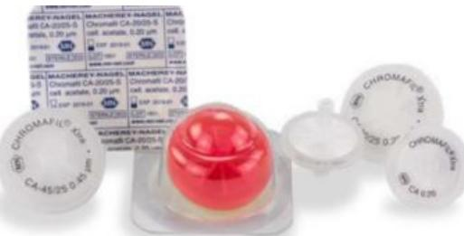
Inside the syringe filter polyester (polyethylene terephthalate) is used as membrane material. The hydrophilic multipurpose PET membrane is suitable for polar as well as nonpolar solvents. It is the HPLC filter, especially suited for mixtures of water and organic solvents. It is not cytotoxic, does not inhibit the growth of microorganisms and higher cells. Labeled for method validation and certification. All CHROMAFIL filters are autoclavable (121 °C and 1.1 bar for 30 min)!
