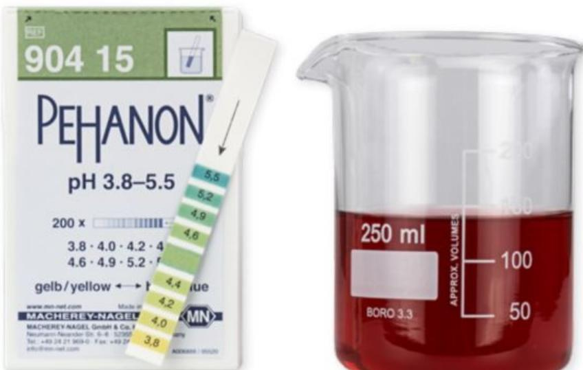
PEHANON test strips unify pH indicator and reference color chart in one strip. Any sample color has the same effect on both, the reference colors and the reactive pad, allowing unadulterated pH reading even in colored solutions.
