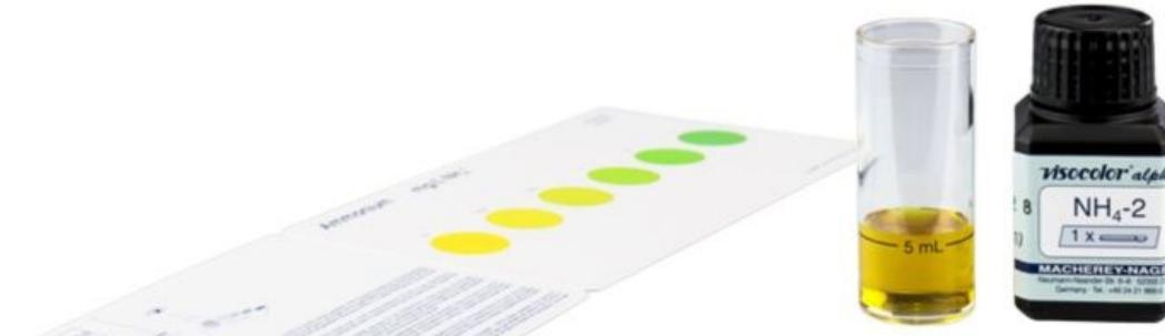
VISOCOLOR alpha is the most simple version of colorimetric and titrimetric test kits. These tests are suitable for visual evaluation only and are very convenient in performance, because of multicomponent reagents. Therefore, test kits are limited in precision and accuracy but represent an inexpensive method for screening tests.
