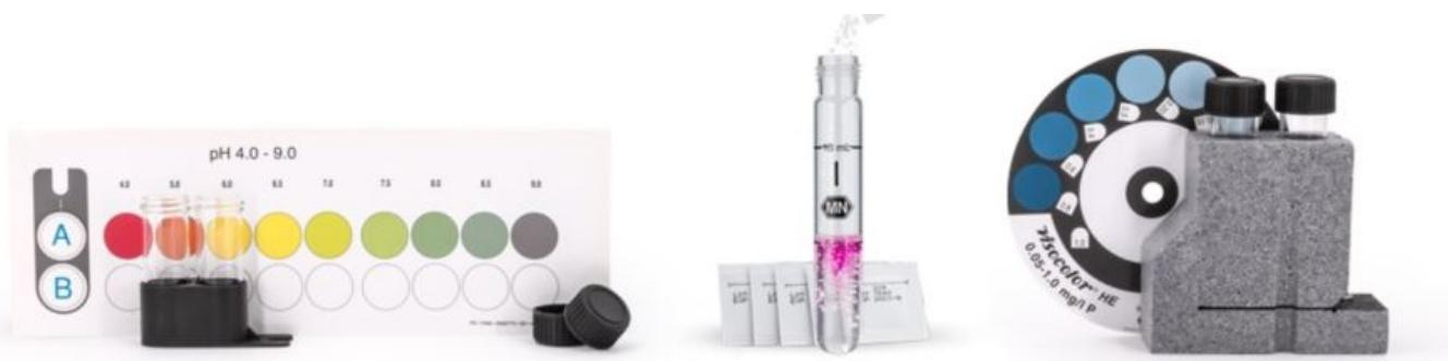
Visual test kits can be evaluated by eye, without further equipment. They are divided into colorimetric test kits, which are compared to a color chart, and titrimetric test kits, where the amount of used reagent is related to the measured value. Some tests are also suitable for photometric evaluation.
