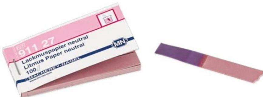
Qualitative pH papers without color chart are simple, completely impregnated indicator papers. Unisol indicator solutions are used for pH determination in pure water, surface waters and very dilute acids or bases.
